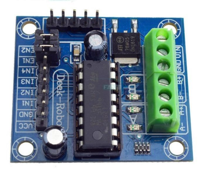
Motor Drive Shield Expansion Board L293d Datasheet
